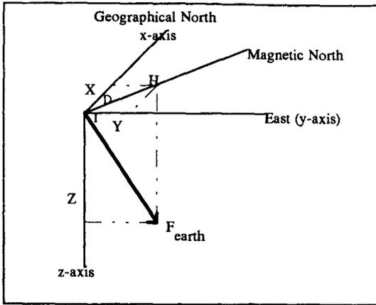
**Figure 3.1.:** Components of the Earth's magnetic field.
