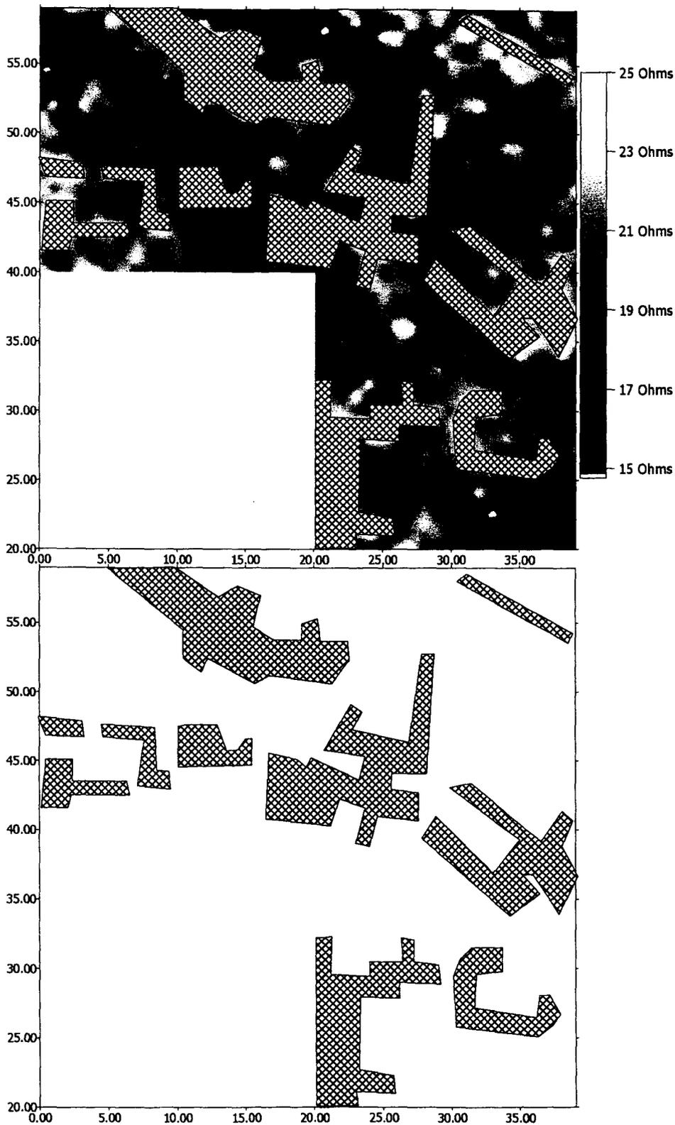
*Figure 5.21:* Diagrammatic representation of the soil resistance anomalies, which have been identified at the site of Perdikaria.
