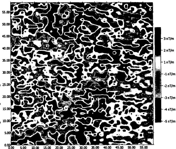
*Figure 5.15:* Colour-scale maps representing the compression of the dynamic range of the magnetic measurements taken at the site of Perdikaria.
