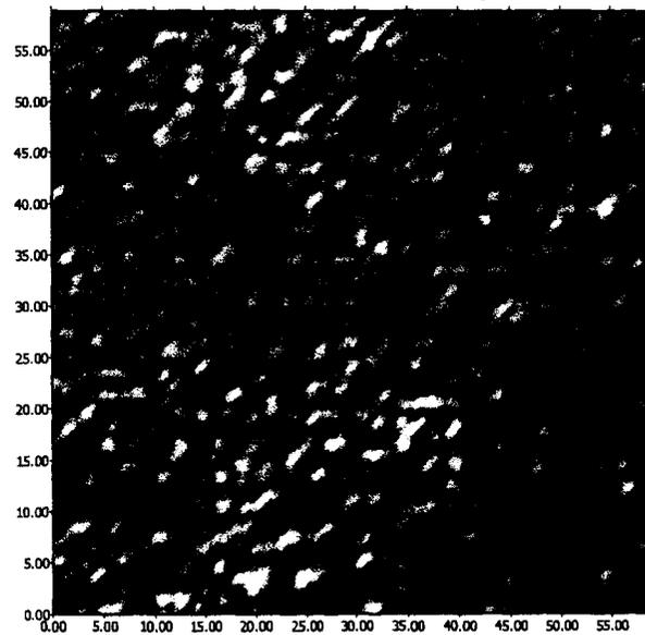
*Figure 5.16:* The application of directional derivatives (in 4 different directions) emphasized a number of linear features in the magnetic map.
