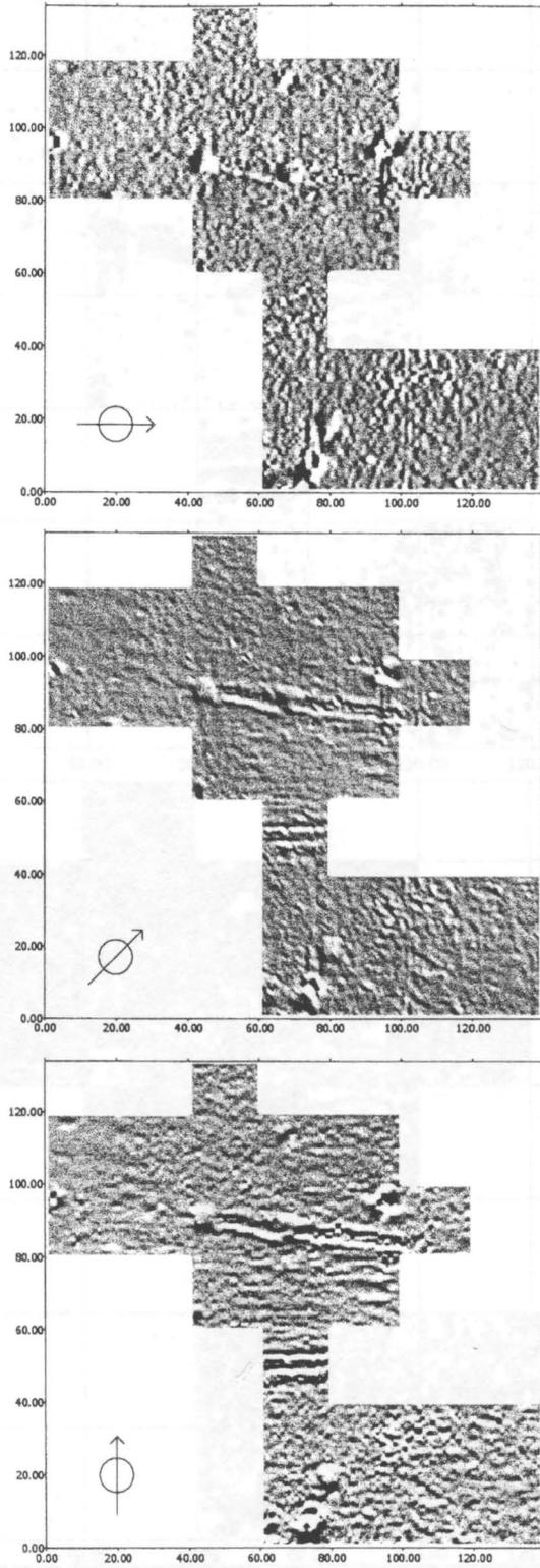
Figure 5.5: Results of the application of directional filters in the direction of 0, 45 and 90 degrees with respect to the East.
