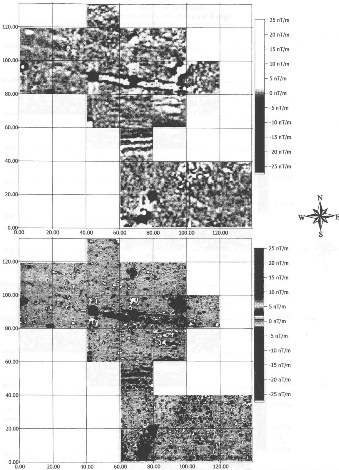
Figure 5.3: Rectification of magnetic measurements to a common level base line. Grey scale and colour scale maps.
