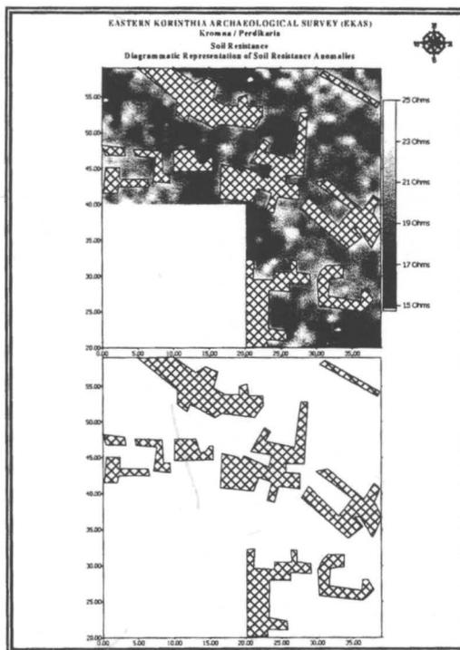
Figure 5.21: Diagrammatic representation of the soil resistance anomalies, which have been identified at the site of Perdikaria.
