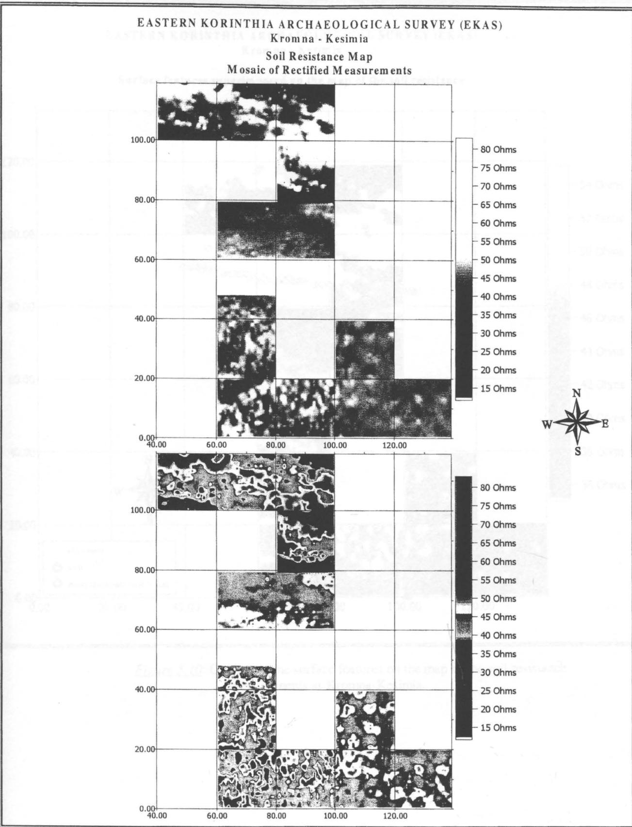
*Figure 5.9:* Mosaic of the rectified soil resistance measurements at Kromna-Kesimia.
