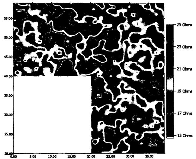
Figure 5.20: Colour-scale maps representing the compression of the dynamic range of the soil resistance measurements taken at the site of Perdikaria.
