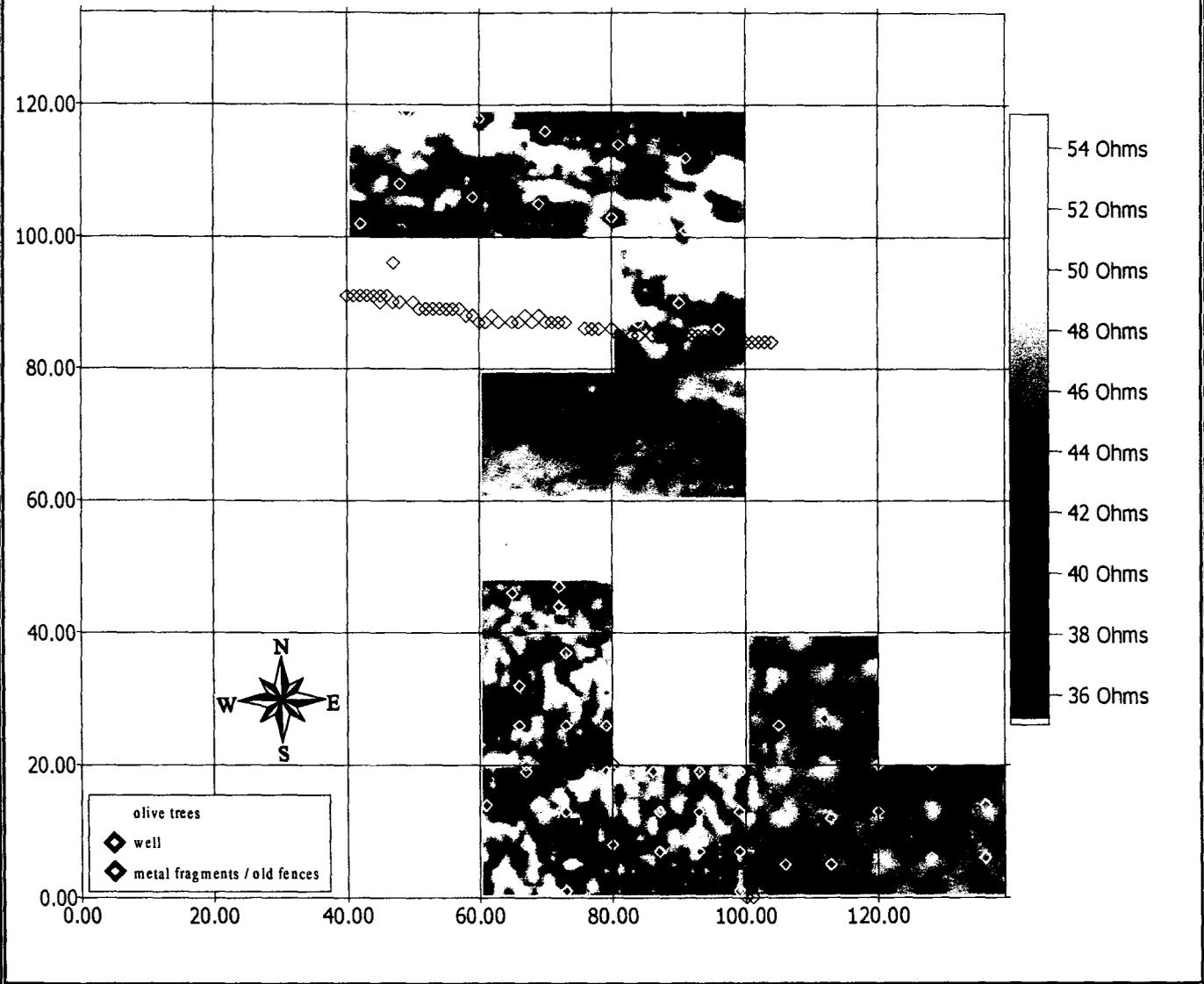
Figure 5.10: Overlay of the surface features on the map of the soil resistance measurements at Kromna-Kesimia.
