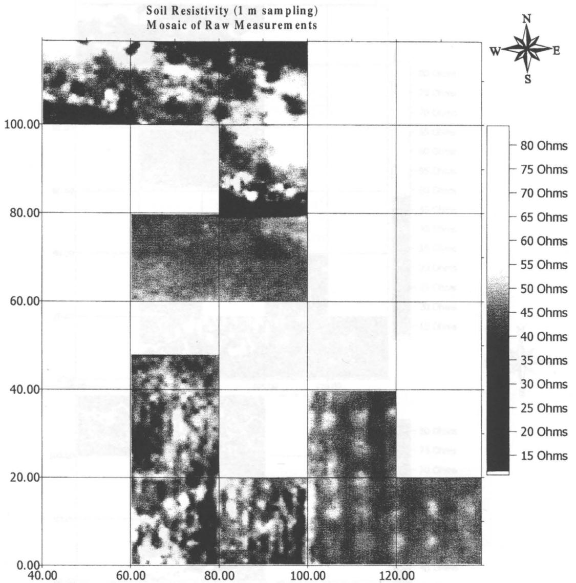
Figure 5.8: Mosaic of the initial soil resistance measurements at Kromna-Kesimia.
