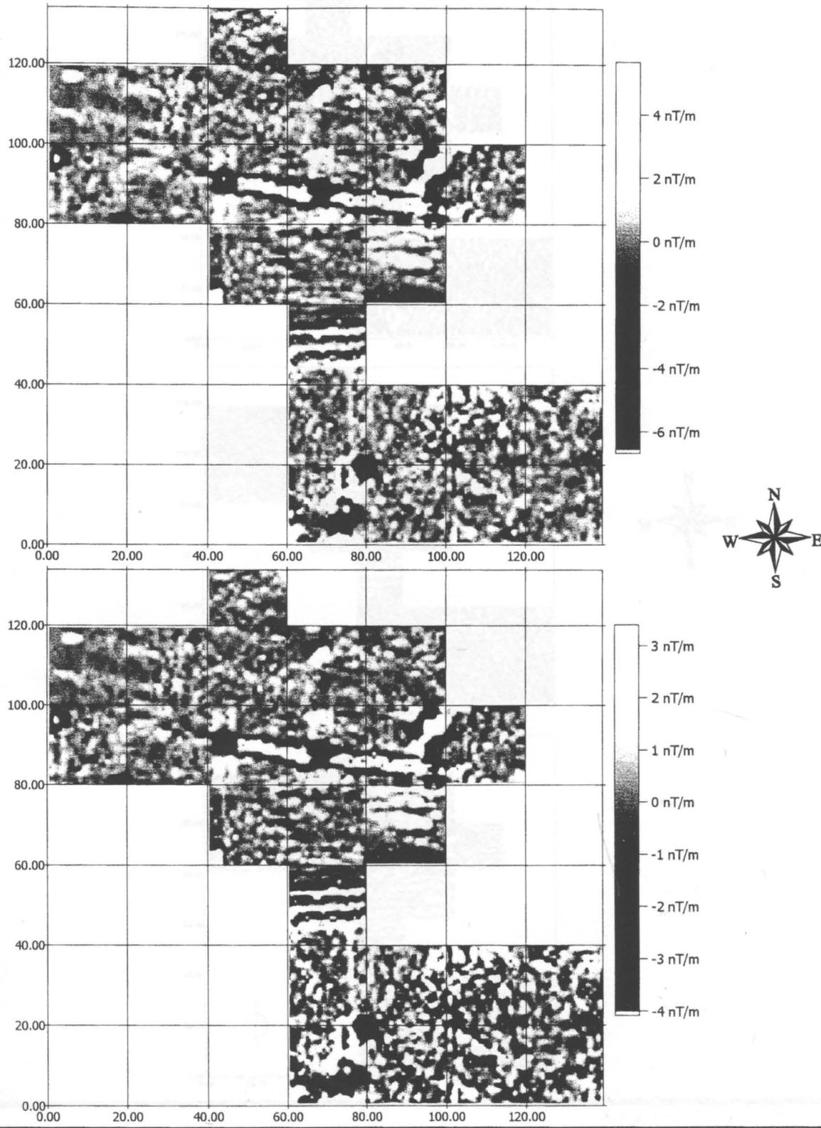
Figure 5.4. Grey scale maps resulting from the compression of the dynamic range of the magnetic values.
