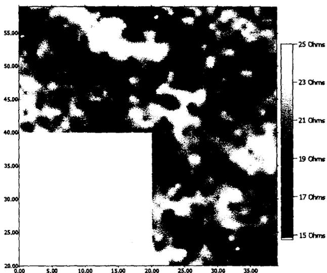
*Figure 5.19:* Grey-scale maps representing the compression of the dynamic range of the soil resistance measurements taken at the site of Perdikaria.
