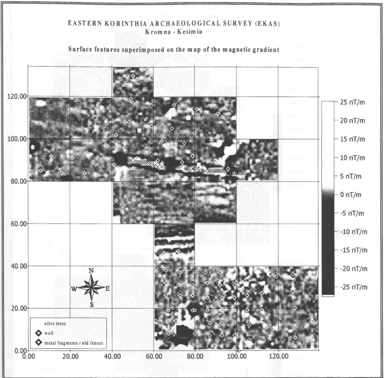
*Figure 5.2:* Overlay of the surface features on the rectified map of the magnetic data. The correlation of some strong anomalies with the existence of old fences, metal fragments and trees is obvious.
